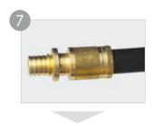
Inspect every joint to ensure the process is correct and complete. The sleeve must be square with the fitting. The joint must be fully compressed.
