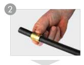
Slide the jointing sleeve over the pipe end with the internal tapered end of the sleve facing the joint. Keep the sleeve at least 50mm from the pipe end.
