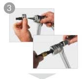
Inspect the expander tool and expander heads prior to use for damage or dirt build up on the heads. Do not use if damaged or missing parts.
